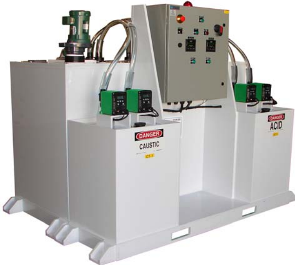
Shown: OMEGA-10-2-B-T-R-1, 10 gpm system, 2 reaction stages, acid and caustic addition, chemical day tanks, 120 VAC relay based control
