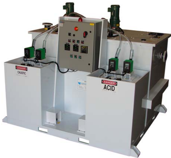
Shown: OMEGA-20-2-B-T-R-1, 20 gpm system, 2 reaction stages, acid and caustic addition, chemical day tanks, 120 VAC relay based control
