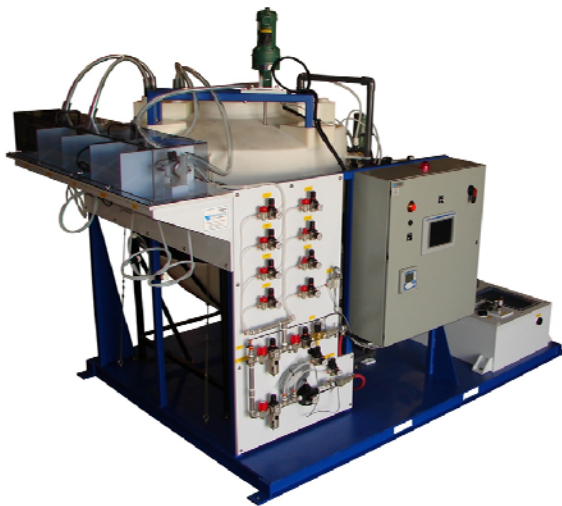
Shown: HMR-NA-500-6FP-M-AB-4-N4-FP 500 gallon reaction tank with a 6 ft 3 filter press, metering pump shelves, and post treatment pH adjustment.
